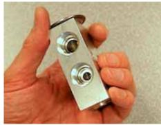
If none of these tests causes the low-pressure gauge needle to rise or drop, the expansion valve is probably defective.
